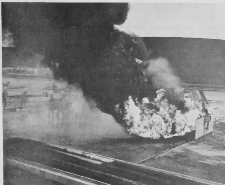
This upwind attack is necessary to move in and close an 8-inch valve that is engulfed in flames.
